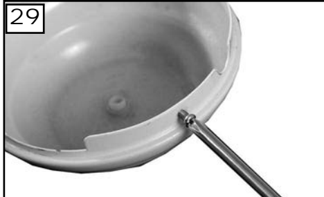
Remove 3 screws on the ridge of the switch cap and save.
