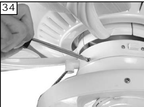
Attach switch cap to fan by lining up 3 screw holes and installing the 3 screws removed and saved from earlier step. Tighten screws securely.
