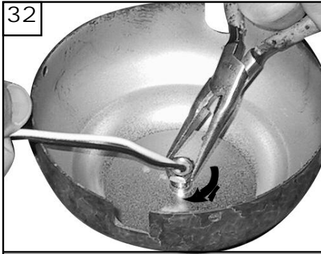
Install keeper nut from the threaded pipe of the light kit.
